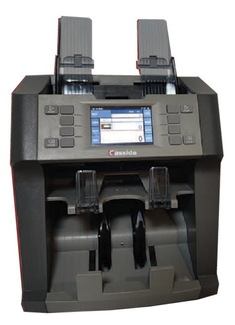
CurencyNumber: 12 Counting Speed: 1000 (Mixed Mode)/1500(Count Mode) Hopper/Stacker: 500-1000/200 Rejecting Capacity Bill: 200 Operating Modes: Mix/Sort/Count/Face/Orientation/Fitness Count eror detections: DBL, HLF, Chain, SD Counterfeit detections: UV/MG/MT/IR/Dual CIS Reports on the display: Auto currency recognition/All currency mixed mode Display type: Color LCD Touch Screen Conection Port: Android Port, LAN Port, RS232/USB/CTP Pit
